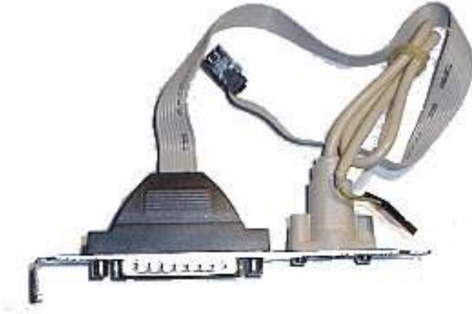
If you are installing ports on the metal insert, you can now screw these inserts into one of the available slots on the back of the case. It is best to choose a slot near the top that will not be used for anything else and provides a short enough distance so that the I/O cables can reach the motherboard.
